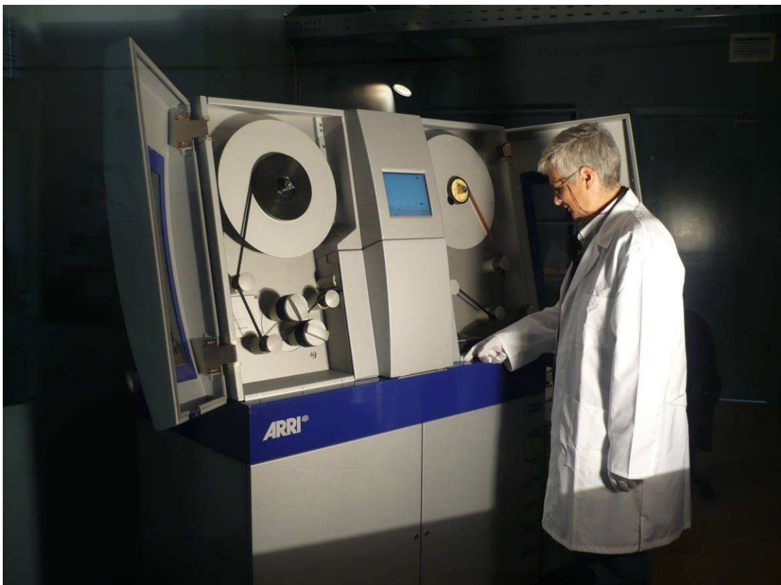
Films are being transferred to digital media after scanning frame by frame.
