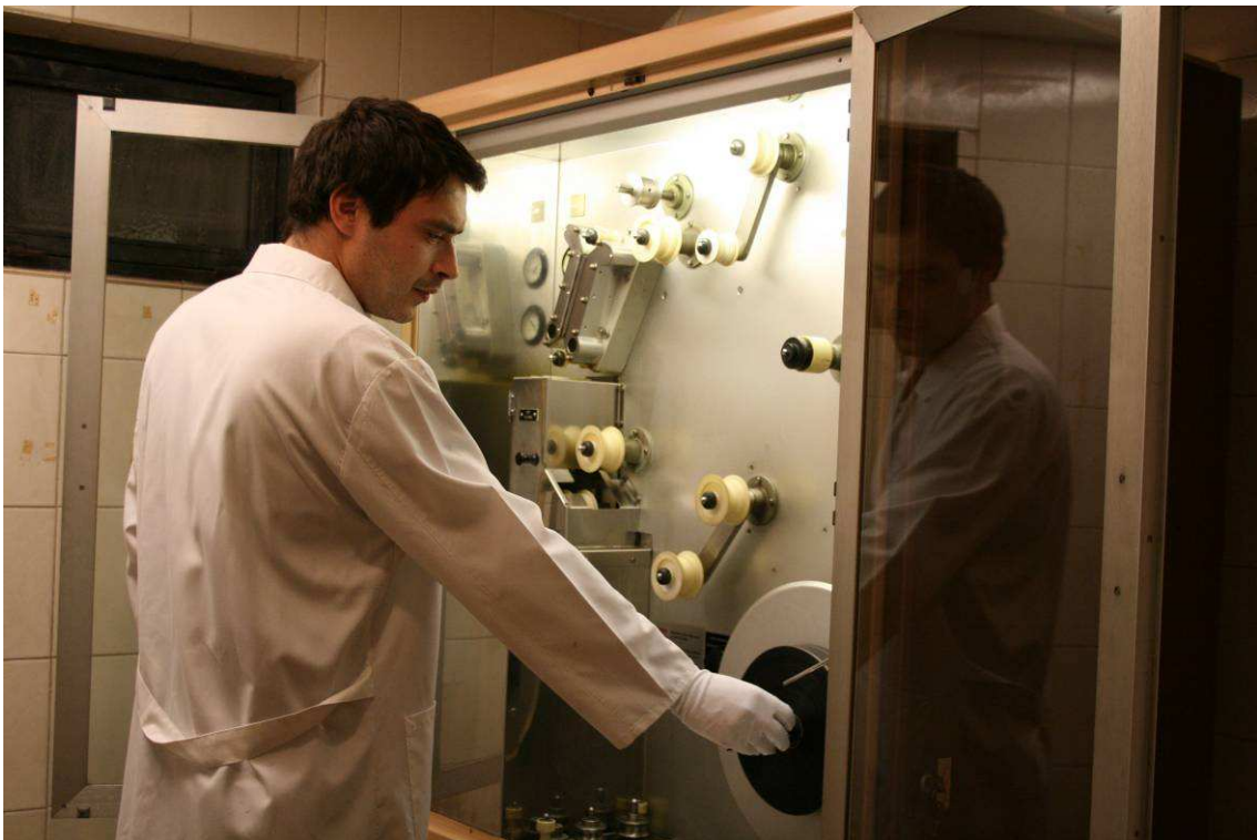
Films are being cleaned by a special solvent and being purified from grease and dust.
